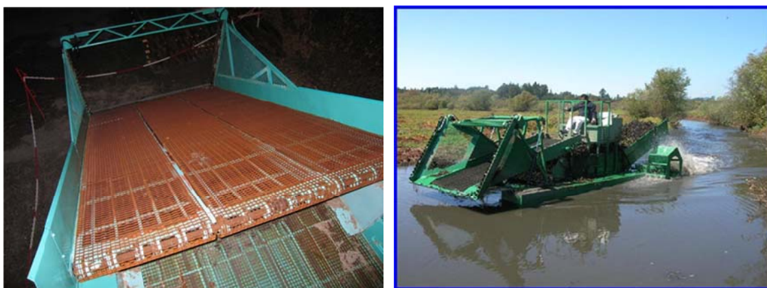
Fig. 4.1 Harvest boat at Zürich See (left) and mechanical harvester from CleanLake Inc. in the USA (right) for bioremediation.
